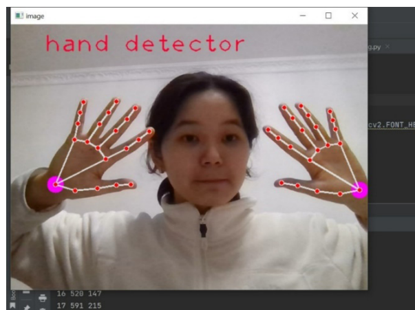
Figure 3 – The first step of the program (hand recognition)
